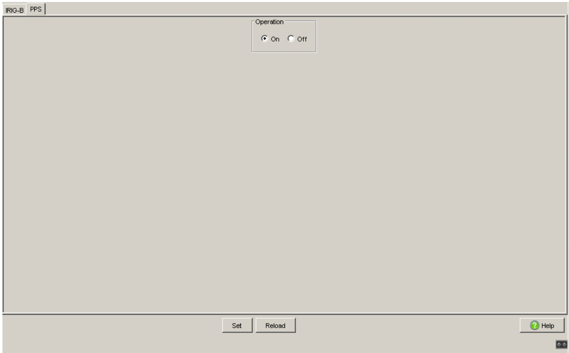
Figure 56: Time > IRIG-B/PPS dialog, "PPS" tab.
